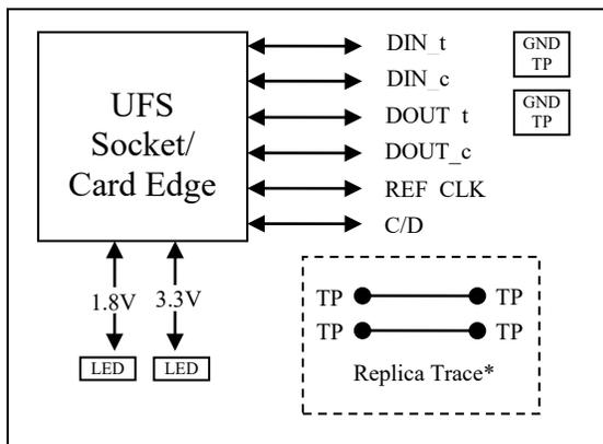
\* The Replica Trace is used to de-embed the test fixture
