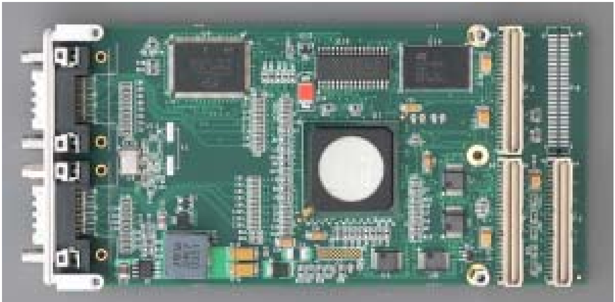
Figure 9: A3803-PMC-05 Host Adapter Configuration
