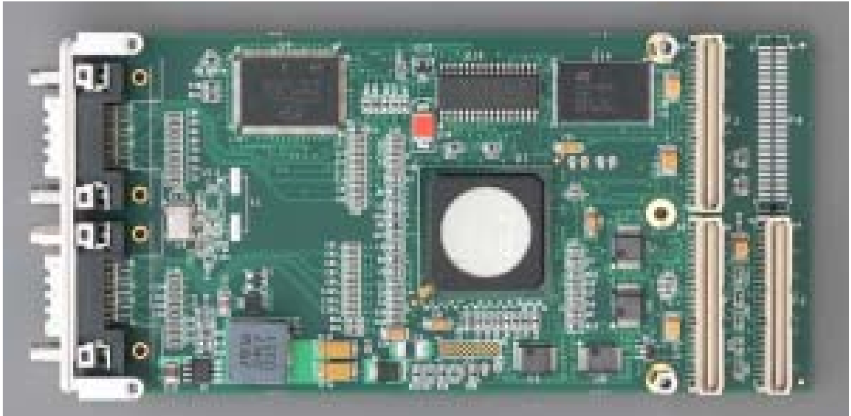
Figure 7: A3803-PMC-04 Host Adapter Configuration
