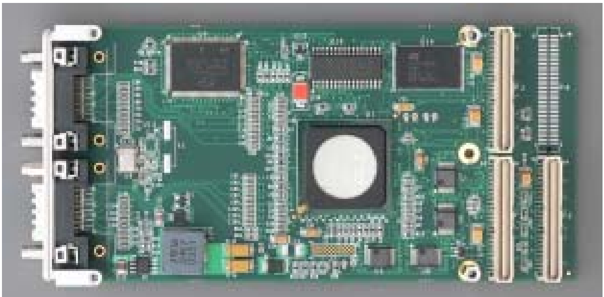
Figure 5: A3803-PMC-01 Host Adapter Configuration
