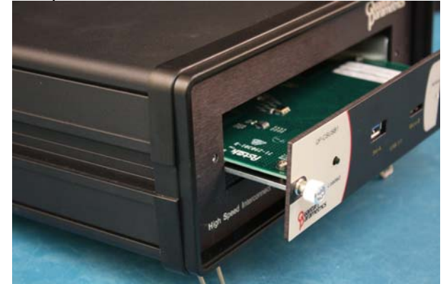
Figure 2—Connector Saver Module and HSIT device
