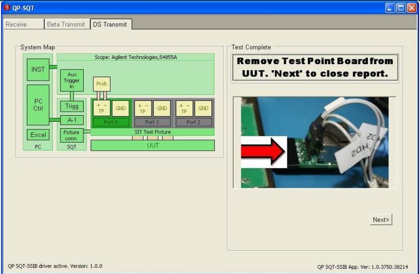
**Figure 16 - Remove test point board**
