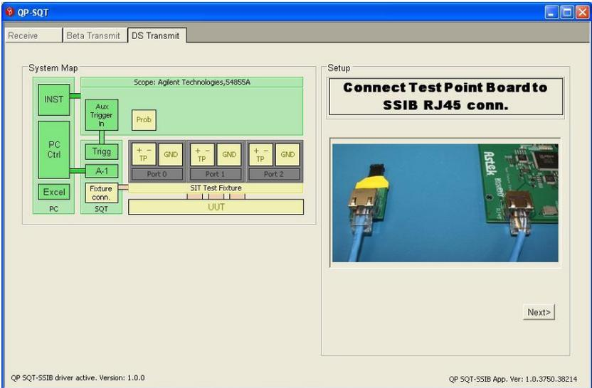
Figure 6 - Test fixture connection
