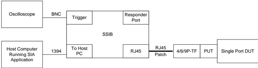
**Figure 2 - Transmit Test Connection diagram (Single Port DUT).**
