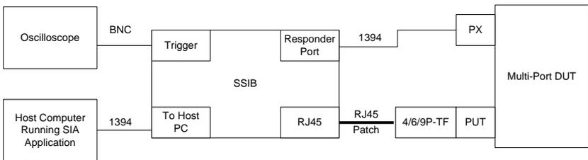
**Figure 3 - Transmit Test Connection diagram (Multi-Port DUT).**
