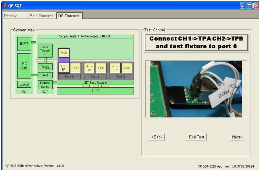
Figure 11 - Connection of probe for testing
