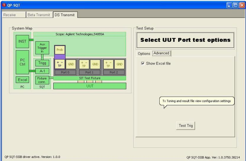
Figure 10 - Advanced transmit test options
