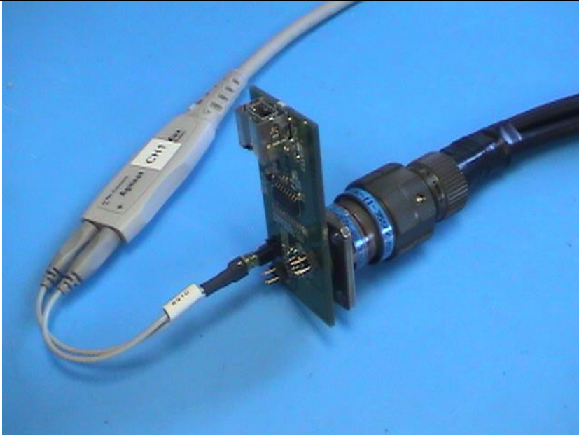
Figure 36 - C-1 Far End signal amplitude measurement.
