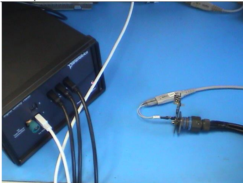
Figure 35 - SQT to 38999 Far End test fixture setup.
